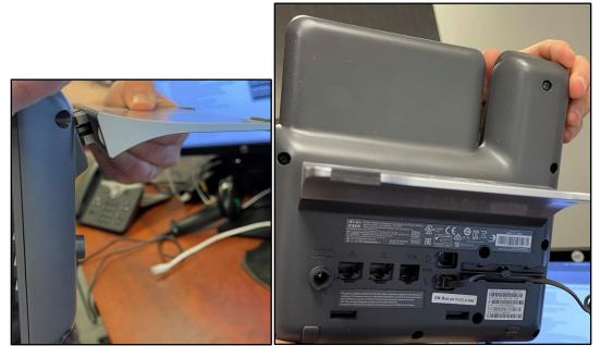
• Plug power cable to injector and insert both Ethernet cables.
