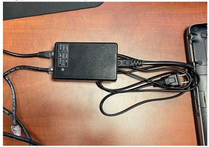
• The cable under the phone icon goes to your phone and the cable under the two connecting computers goes to your Router/Modem.
